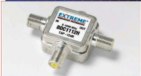
Model BDC1100H 1-Output Broadband Digital Directional Coupler, 1GHz Tap Values: 04, 06, 09, 12, 16, 20, 24, 27, 30 dB
